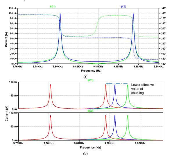
**Figure 2.** (a) Frequency response of a coupled RLC system for a fixed value of a coupling, magnitude (**left**) and phase (**right**); (b) frequency response of a coupled RLC system for variants of effective coupling. Lower coupling leads to closely-spaced mode frequencies.
