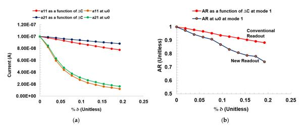
**Figure 5.** Output response of a coupled RLC capacitance readout circuit. (**a**) Output current amplitude vs.  $\Delta C$  or  $\delta$ . Lable a11 is amplitude of resonator 1 at mode 1, a22 is amplitude of resonator 2 at mode 1 (**b**) Amplitude ratio (AR) readout of RLC coupled resonator circuit.  $\omega_0$  is the initial readout resonant frequency at mode 1.
