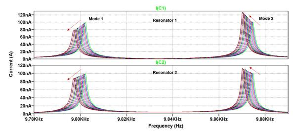
**Figure 3.** Frequency response of a coupled RLC capacitance sensor system. Top plot shows response of resonator 1 and bottom plot shows response of resonator 2. Direction of arrow indicates a variation trend of the resonant peak of the jth (j = 1, 2) resonator at the ith (i = 1, 2) mode of the frequency response.
