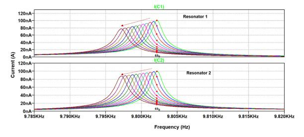
**Figure 4.** Frequency response of a coupled RLC capacitance readout system. Response of resonator 1 (**top**) and response of resonator 2 (**bottom**). Direction of dotted line indicates measuring a proposed variation trend of the resonant peak of the jth (j = 1, 2) resonator at the ith (i = 1, 2) mode of the frequency response. Shown here is the output response of the jth (j = 1, 2) resonator at the first mode of a coupled RLC resonant capacitance readout.
