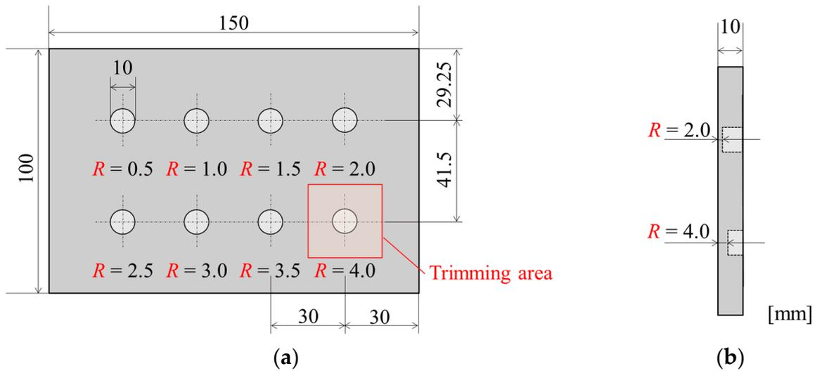
**Figure 1.** Flat-bottom hole specimen employed in this study: (a) illustration of the specimen of the side for infrared temperature measurement; (b) illustration of cross-section of (a).
