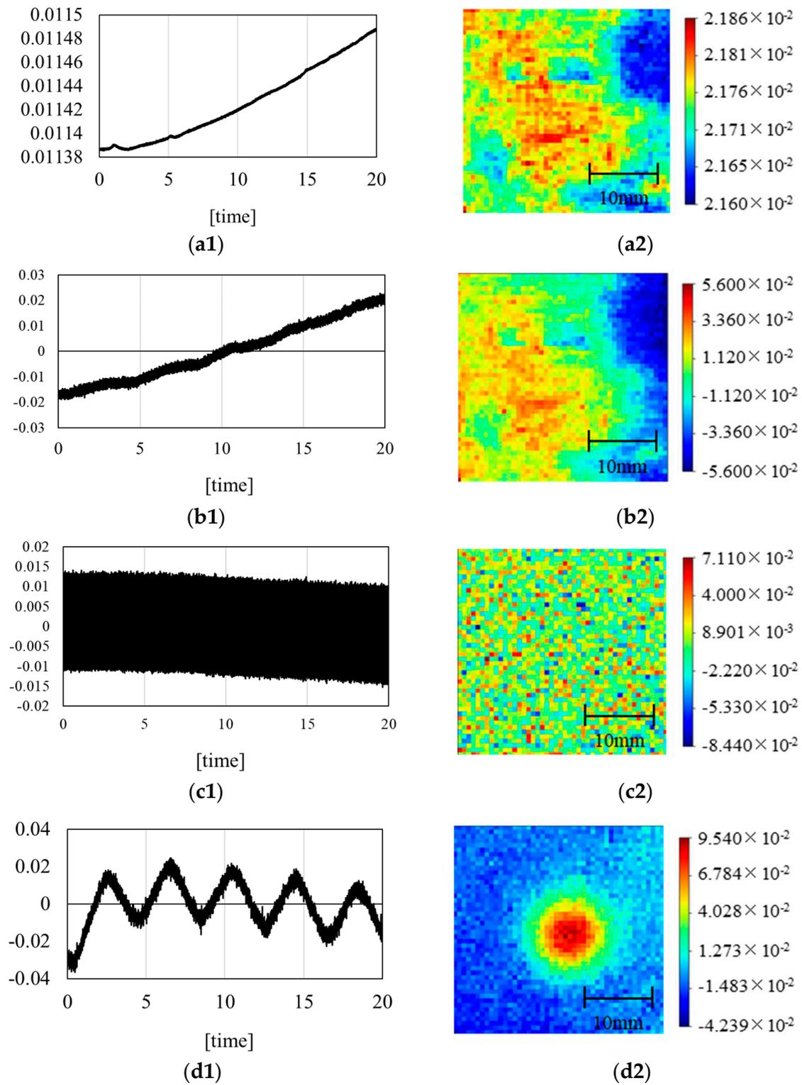
**Figure 2.** Results of the SVD thermo-component analysis of thickness  $R = 4.0$  mm: (a1) PC1, (b1) PC2, (c1) PC3, and (d1) PC4 time-series temperature variation waveform; (a2) EOF1, (b2) EOF2, (c2) EOF3, and (d2) EOF4 images of the relative value distribution image with PC waveform.
