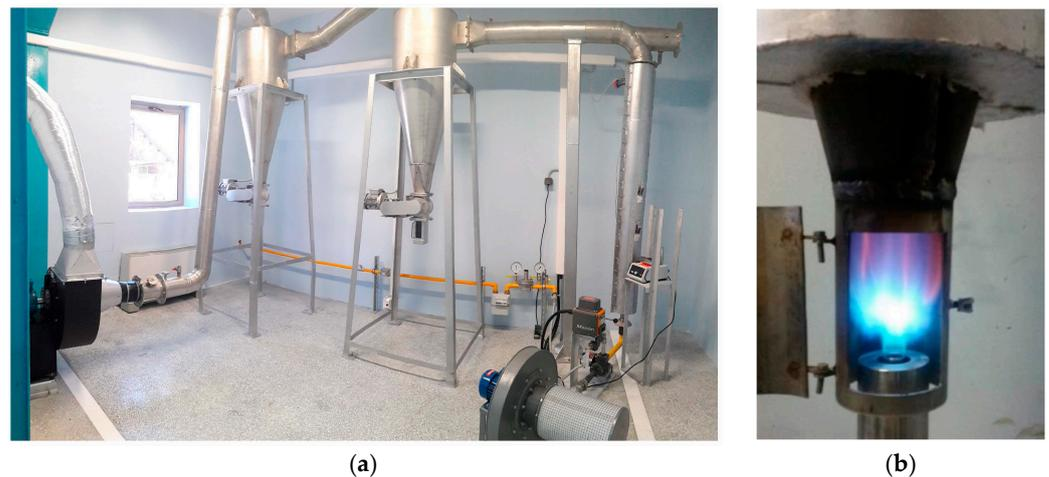
**Figure 1.** Vertical lab perlite-expansion furnace operating with LPG. (a) Furnace. (b) Module for expanding ultrafine grades.
