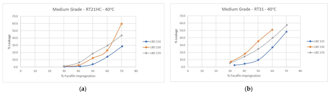
**Figure 5.** Leakage tests of PCM composites prepared by impregnating medium-grade expanded perlite at different densities in paraffin (a) RT21HC and (b) RT31.
