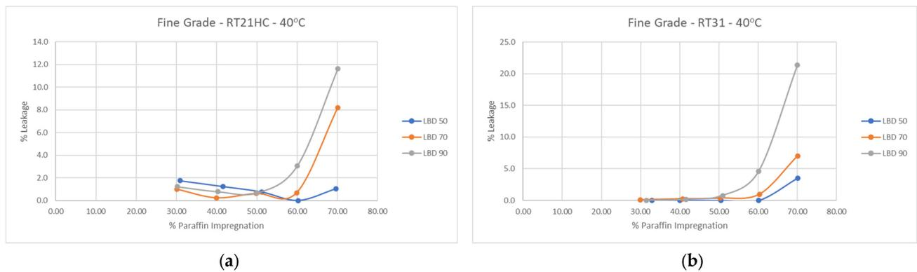
**Figure 4.** Leakage tests of PCM composites prepared by impregnating fine-grade expanded perlite at different densities in paraffin (a) RT21HC and (b) RT31.
