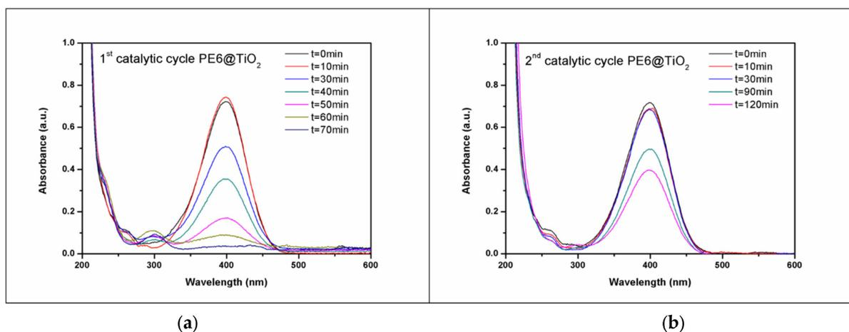
**Figure 3.** Spectra of 4-nitrophenol reduction to 4-aminophenol in the presence of the  $\text{PE6@TiO}_2$  photocatalyst under sunlight exposure for one (a) and two (b) process cycles.
