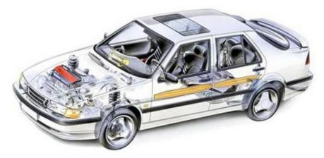
Figure 1. First use of hot stamping on a production car. Saab 9000. Side impact beam [2].
