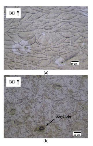
**Figure 3.** Example of transition from conduction melting to keyhole formation. (**a**) Optical micrograph of the longitudinal section to the build direction (BD) of S1-FeSi6.5 sample ( $E = 150 \text{ Jm}^{-1}$ ,  $v = 0.5 \text{ ms}^{-1}$ , P = 75 W), conduction melt mode. (**b**) Optical micrograph of the longitudinal section to the build direction (BD) of S18-FeSi6.5 sample ( $E = 350 \text{ Jm}^{-1}$ ,  $v = 0.5 \text{ ms}^{-1}$ , P = 175 W), keyhole mode
