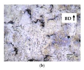
**Figure 4.** (a) Example of columnar microstructure of longitudinal sections along the built direction (BD) of the highest density samples (S7-FeSi3,  $E = 250 \text{ Jm}^{-1}$ ,  $v = 1 \text{ ms}^{-1}$ , P = 250 W). (b) Example of non-columnar microstructure in a high porosity samples (S1-FeSi3,  $E = 150 \text{ Jm}^{-1}$ ,  $v = 0.5 \text{ ms}^{-1}$ , P = 75 W).
