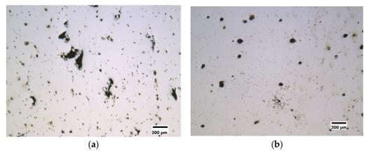
**Figure 1.** Specific laser energy effect E [Jm<sup>-1</sup>] on the densification of FeSi3 steel-samples. (**a**) Sample S1 (E = 150 Jm<sup>-1</sup>, v = 0.5 ms<sup>-1</sup>, P = 75 W), relative density of the sample 99.93% and pores with irregular shape. (**b**) Sample S18 (E = 350 Jm<sup>-1</sup>, v = 0.5 ms<sup>-1</sup>, P = 175 W), relative density of the sample 99.98% and pores with spherical shape.
