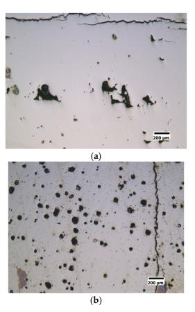
**Figure 2.** Specific laser energy effect E [Jm<sup>-1</sup>] on the densification of FeSi6.5 steel samples. (a) Sample S1 (E = 150 Jm<sup>-1</sup>, v = 0.5 ms<sup>-1</sup>, P = 75 W), relative density of the sample 99.93% and pores with irregular shape. (b) Sample S18 (E = 350 Jm<sup>-1</sup>, v = 0.5 ms<sup>-1</sup>, P = 175 W), relative density of the sample 99.98% and pores with spherical shape.
