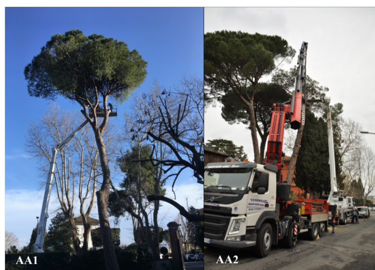
Figure 5. The felling yards AA1 and AA2. Note in the AA2 the truck mounted crane employed to descend the heaviest logs.
