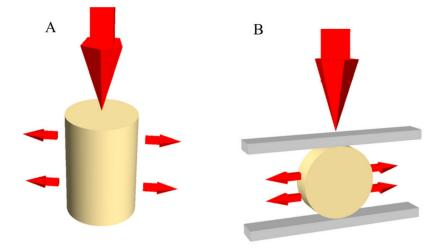
Figure 1. Schematic illustration of: (A) compressive strength test; and (B) diametral tensile strength test.
