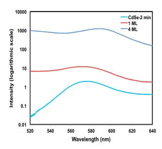
$\begin{tabular}{ll} \textbf{Figure S2.} The PL spectrum of CdSe two-minute aliquot QDs and the core-shell CdSe-ZnO with 1 and 4 MLs of ZnO. \end{tabular}$
