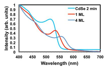
**Figure S1.** The absorption spectrum of CdSe two-minute aliquot QDs and the core-shell CdSe-ZnO with 4 MLs of ZnO.
