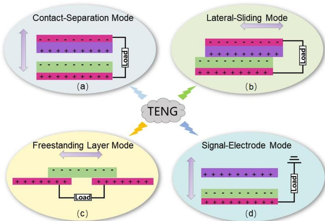
**Figure 2.** TENGs have four distinct working modes. Reprinted with permission from Ref. [63]. Copyright 2022, Springer. (a) Contact-separation mode (CS) [65–67]. (b) Lateral sliding mode (LS) [68–70]. (c) Freestanding triboelectric-layer mode (FT) [73–75]. (d) Single-electrode mode (SE) [71–73].
