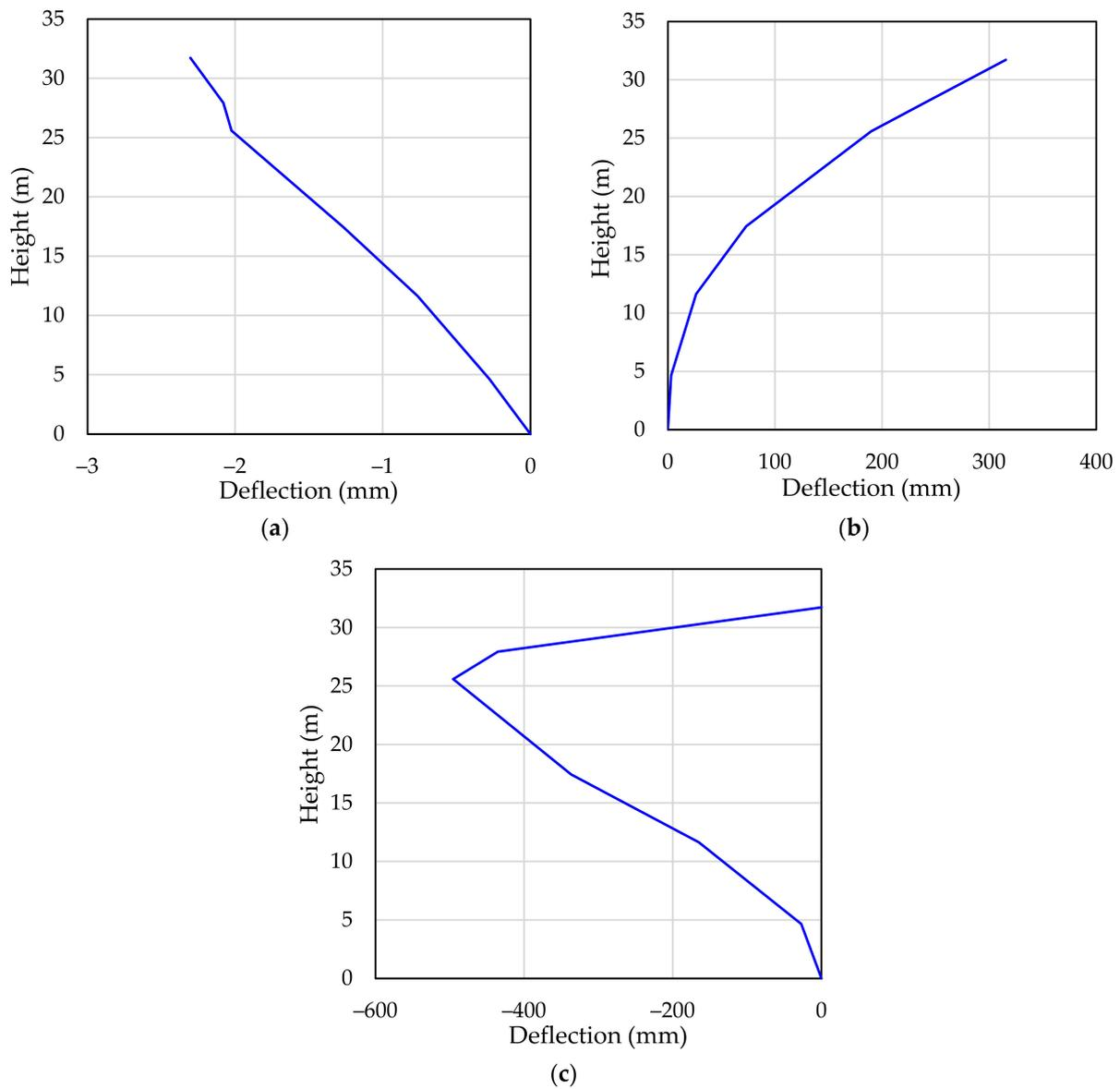
**Figure 5.** Deflections for: (a) vertical direction from load case 1; (b) transverse direction from load case 1; and (c) longitudinal direction from load case 3.
