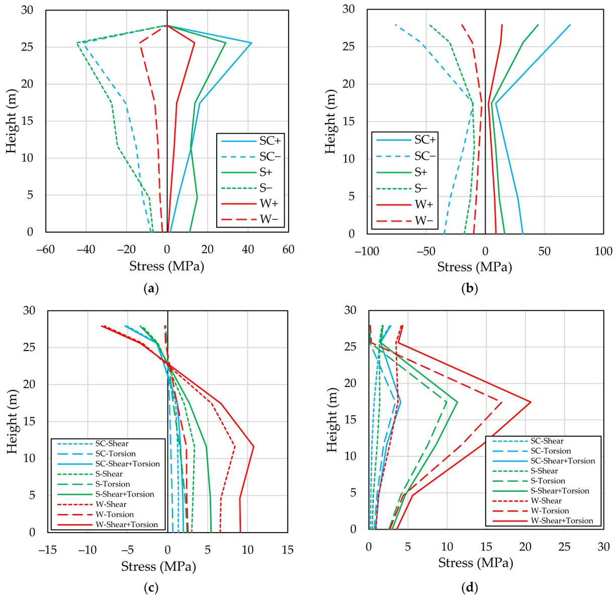
**Figure 4.** Diagrams for: (a) controlling axial stresses from load case 1; (b) controlling axial stresses from load case 2; (c) controlling shear stresses from load case 2; and (d) controlling shear stresses from load case 3.
