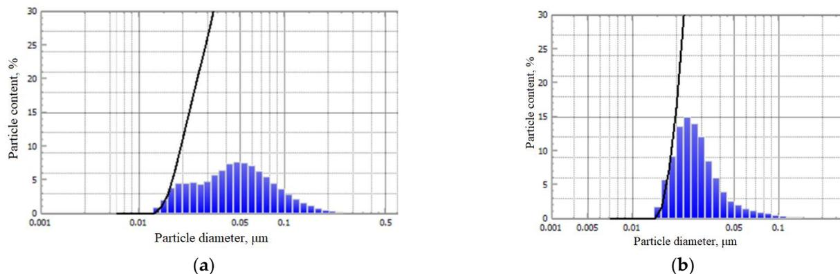
**Figure 4.** Particle size distribution in the chrysotile dispersion after its treatment in a cavitation disperser: (a) freshly prepared dispersion (average size—46 nm); (b) after storage for 2 years (average size—26 nm).
