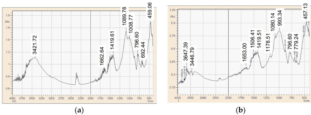
**Figure 6.** IR spectrum of the sample: (a) reference composition; (b) modified with a complex additive based on carbon black and chrysotile asbestos.
