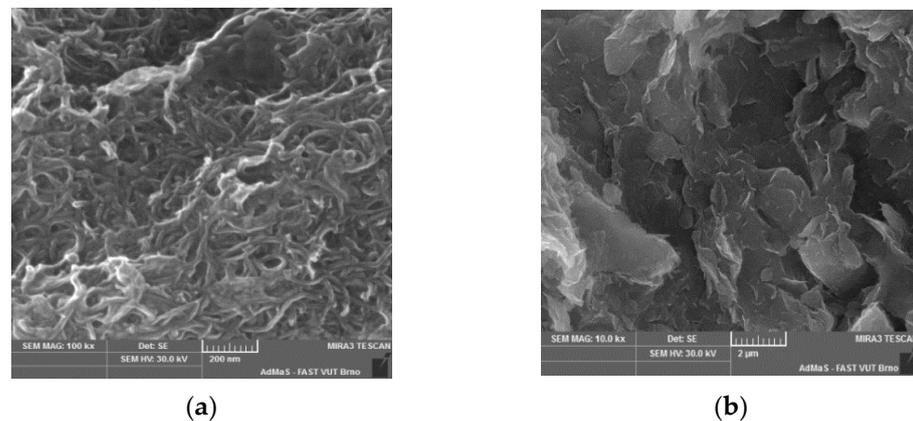
**Figure 1.** Microstructure of: (a) carbon nanotube dispersions with grafted functional groups based on carboxymethylcellulose; (b) carbon black dispersions.
