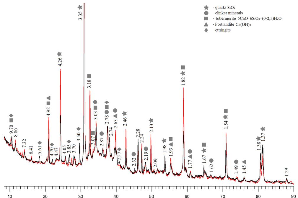
**Figure 7.** Spectra of X-ray phase analysis of the reference composition sample (black) and a sample modified with a complex additive based on chrysotile fibers and carbon black (red).
