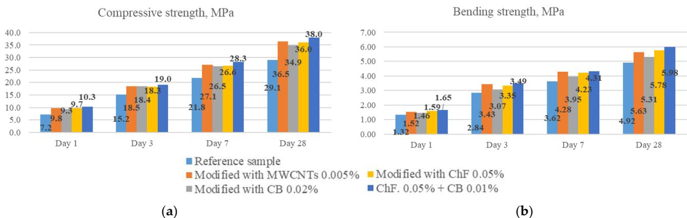
**Figure 3.** The dynamics of the strength development of cement-based compositions depending on the type of additive introduced: (a) in compression; (b) in bending.
