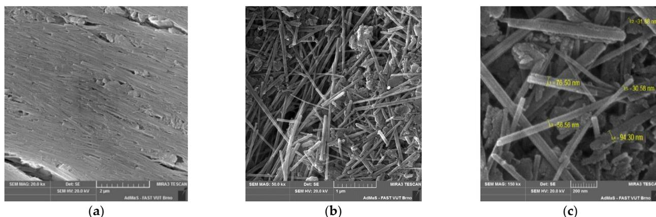
**Figure 2.** Microstructure of chrysotile fibers: (a) before processing, at 20,000-fold magnification; (b) after processing, at 50,000-fold magnification; (c) the same at 150,000-fold magnification.
