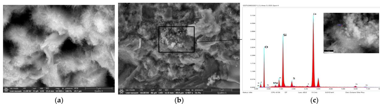
**Figure 5.** Microstructure of the cement composite: (a) reference at 10,000-fold magnification; (b) modified with a complex additive based on carbon black and chrysotile fibers at 6900-fold magnification; (c) X-ray spectral analysis of the hydration products.
