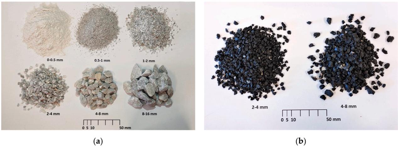
Figure 1. Sieved gradations of the (a) mineral aggregate and (b) rubber particles.
