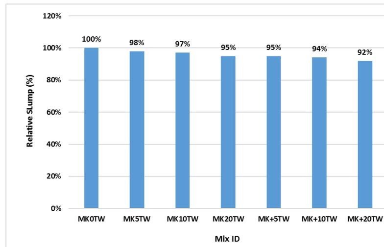
Figure 4. Impact of different ratios of MK on the slump values of concrete mixed with TW.
