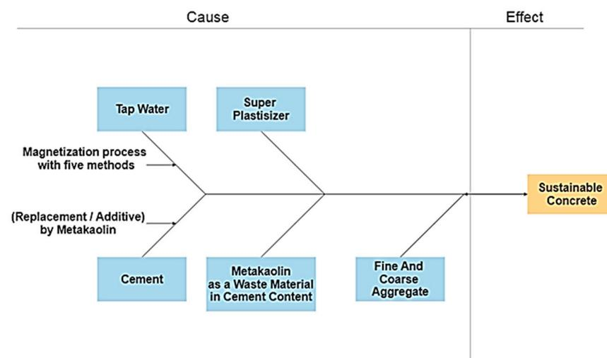
Figure 2. Ishikawa cause-and-effect diagram of producing sustainable concrete utilizing metakaolin and magnetized water.
