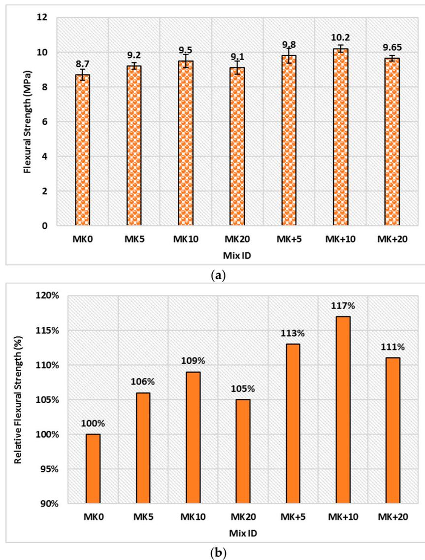
**Figure 7.** Variation in 28-day flexural strength for MK concrete made with TW: (a) values with error bars, and (b) relative change.
