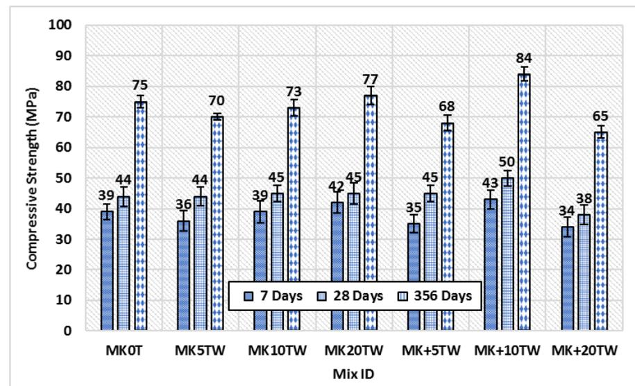
Figure 5. Effect of ratios of MK on the compressive strength of concrete mixed by TW (reprinted from [21]).
