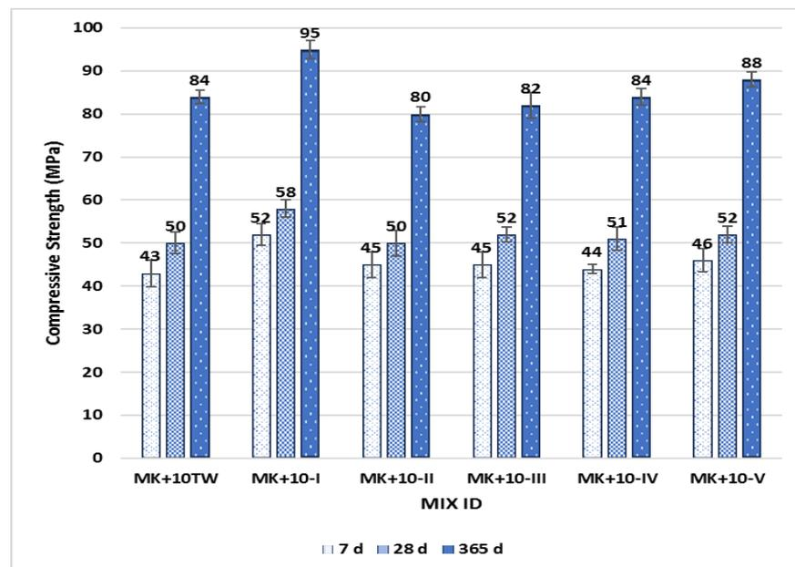
Figure 9. Effect of different methods of water magnetization on MK concrete compressive strength.
