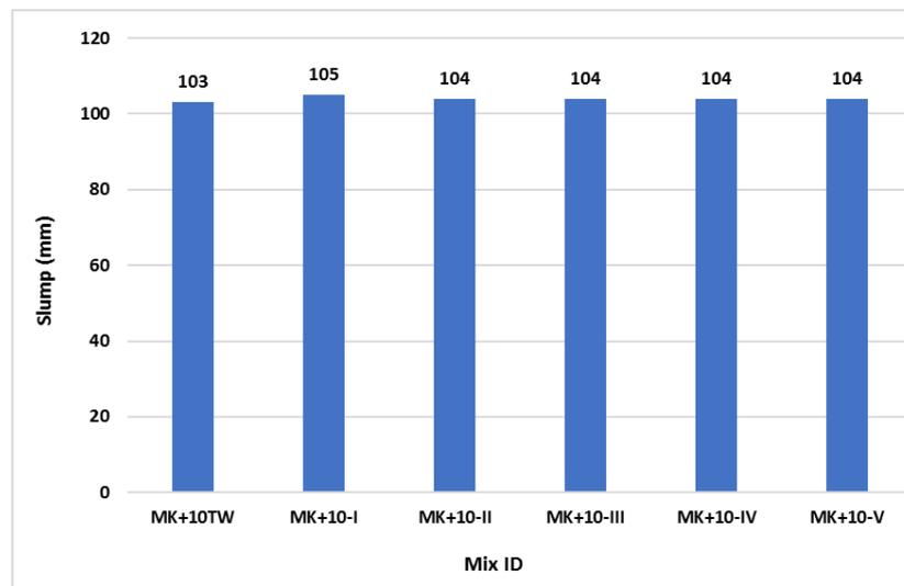
Figure 8. Effect of different methods of water magnetization on MK concrete slump.
