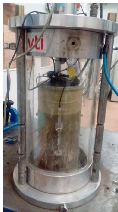
**Figure 4.** Repeated load triaxial equipment used in the study.
