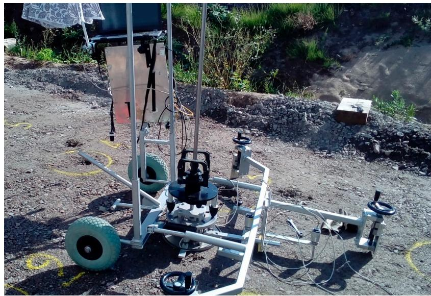
**Figure 2.** The VTI's lightweight deflectometer.
