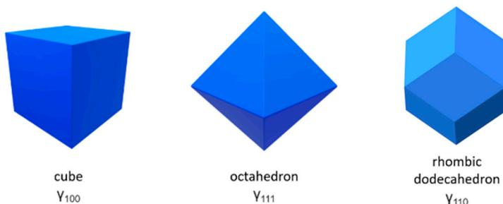
**Figure 1.** Examples of Wulff constructions for shapes of high cubic symmetry.
