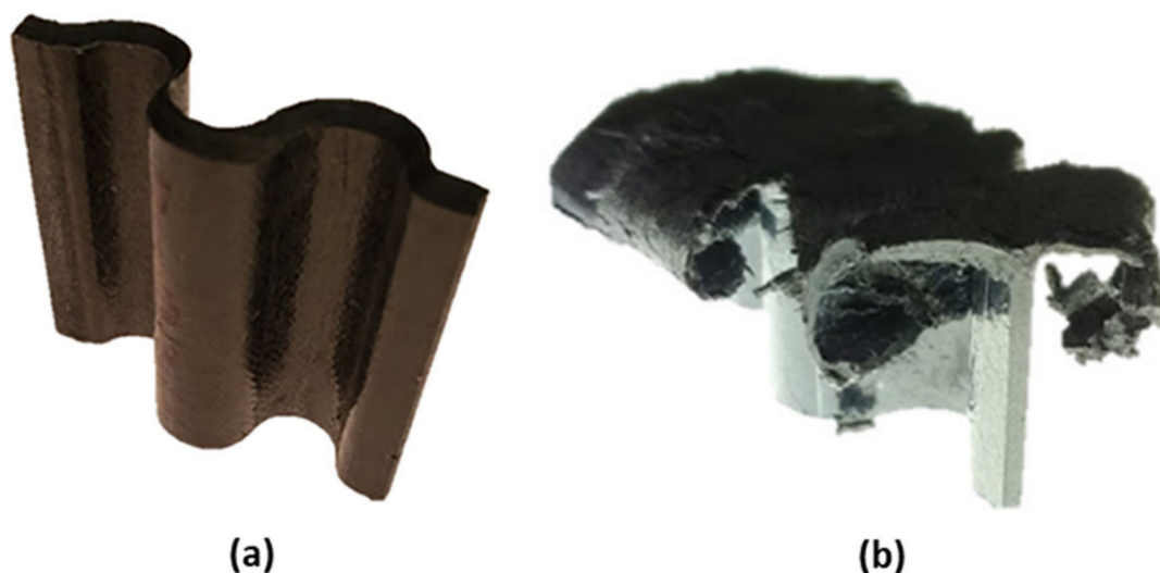
Figure 15. Constant cross-section crush specimens in the sinusoidal geometry: (a) untested sample and (b) failed sample. Reprinted with permission from [88]. Copyright 2021 Elsevier.
