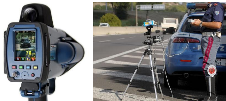
Figure 8. Speed measurement with telelaser, which exploits the high-frequency laser emitted in the direction of passing cars, even when they are at a great distance, effectively making useless the braking that many motorists dangerously do when they see a speed camera.
