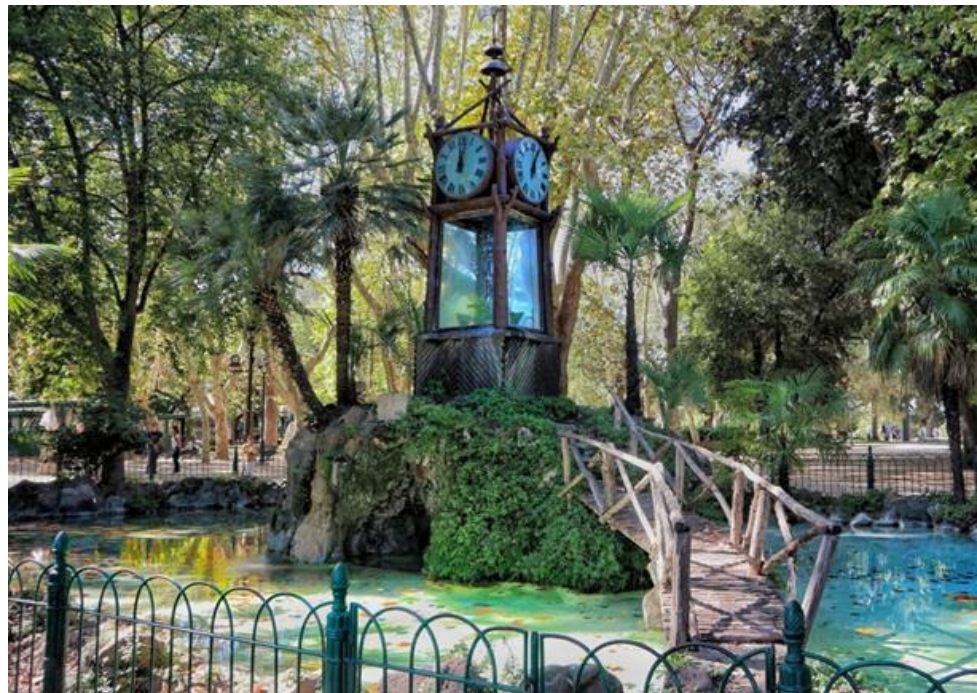
Figure 9. Water clock made in 1867 by Father Giovanni Battista Embriaco and currently exhibited in Villa Borghese in Rome. The movement of the clock hands is caused by the oscillation of two rods connected to two leaf-shaped basins, filled alternately by a jet of water.
