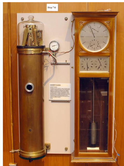
Figure 10. Shortt clock in US National Institute of Standards and Technology Museum, Gaithersburg, Maryland. The primary pendulum (on the left, in its copper vacuum tank) and the secondary pendulum (on the right, linked to the clock mechanism) were synchronized by electro-mechanical means.
