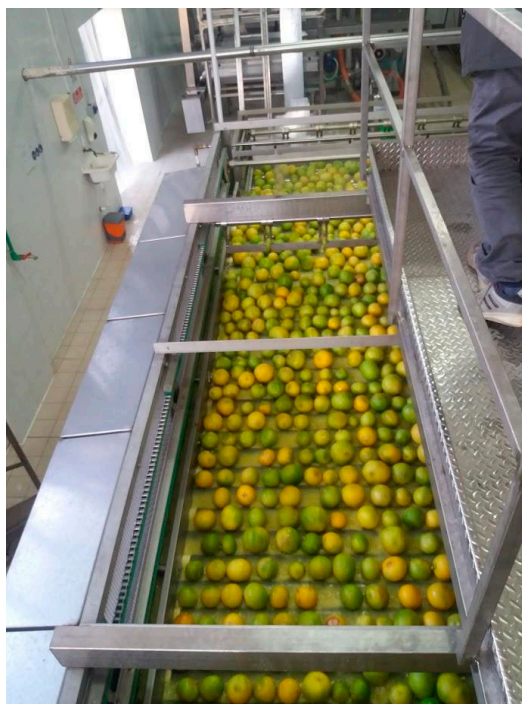
Figure 2. The bed of rolling toothed cylinders in a Garozzo machine.
