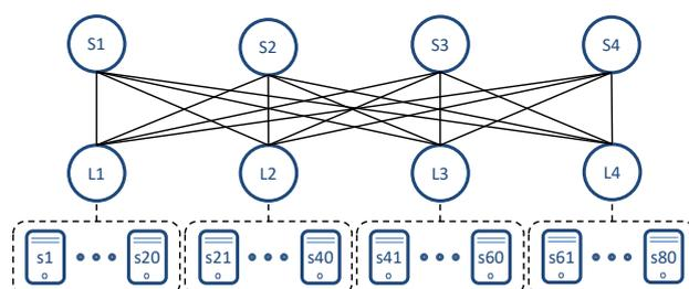
Figure 8. Spine-Leaf topology (parameters  $4 \times 4$ ).
