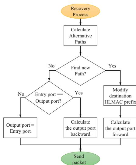
**Figure 6.** Recovery logic in the eTorii implementation.
