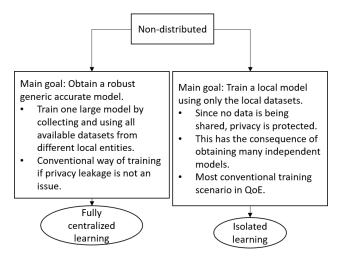
Figure 1. Comparison of conventional Centralized and Isolated Training scenarios.
