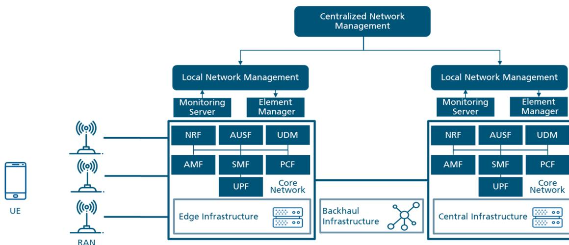
**Figure 2.** Simplified 5G Architecture. The core network functions are depicted twice at edge and at central to illustrate that they can be placed at either location.
