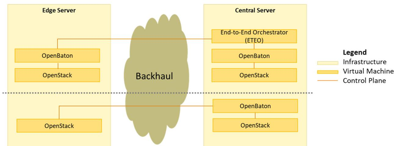
**Figure 6.** Network management testbed implementation.
