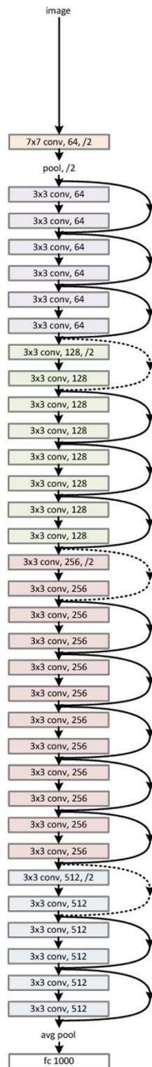
**Figure 1.** Architecture of ResNet-34 network with 34 parameter layers. Curved arrows symbolize identity mapping. Dotted shortcuts represent an increase of the dimensions.
