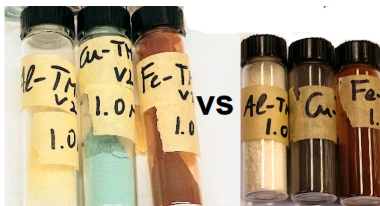
Figure S1. Visual difference between the prepared materials with careful (left) neutralization step for successful materials preparation vs. metal oxide precipitation and lack of metal incorporation into the framework (right).
