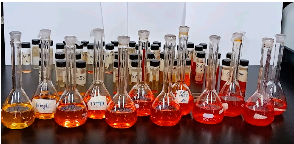
Figure S3. Adsorption isotherm studies with methyl orange. Starting solutions in the foreground while Al-TMC-N and Cu-TMC-N (Fe-TMC-N not shown for clarity and lack in visual difference) are after adsorption. Solutions from 10-1000 mg/L were tested.
